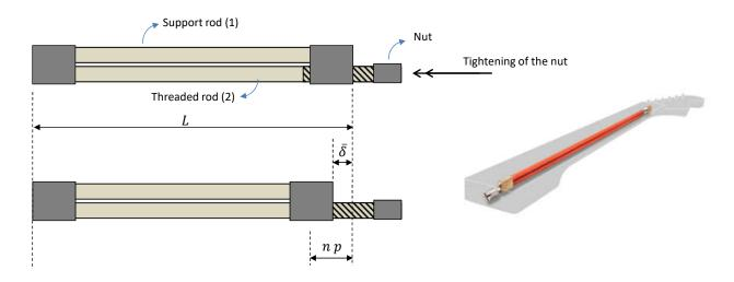
We must understand the resulting geometry and deformation when the nut is tightened. Let us assume that the left end of the rod is fixed.
